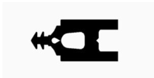
AE055 – Thermal Break. Please see Aluminium Gaskets & Pressure Plates for complete range. (Scale 1:1)
