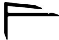
ESEC – Small external corner 2mm – 3mm boarding. (Scale 1:1)
