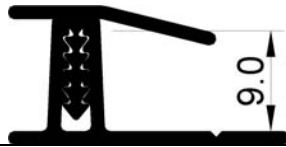
ETPE9/15T (top part) & ETPE9/15B (bottom part) – Two part adjustable edge strip. 9mm – 15mm boarding. (Scale 2:1)
