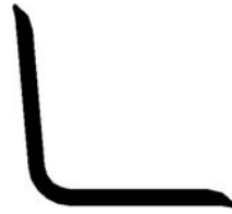
L25A95 – 25mm Internal Angle (Scale 1:1)
